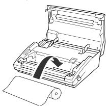
Pull out the paper edge from the edge of the fax machine as shown.
